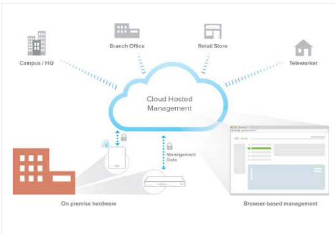
Cisco Meraki Cloud Management Architecture
